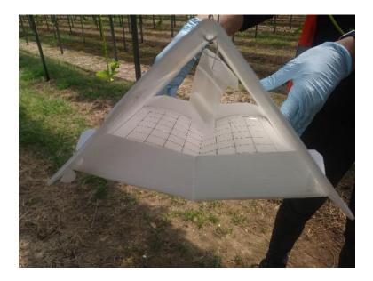
**Figure 3.1.6**. White Delta Trap® with sticky insert in the base during Trial 1 of the aphidophagous hoverfly trial 2022.
