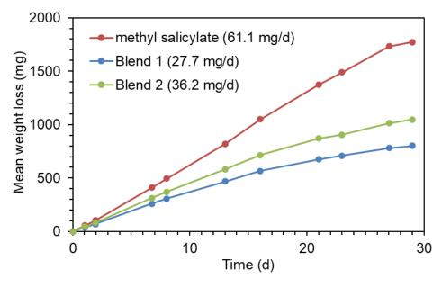
**Fig. 3.1.8.** Release rates from NRI sachets measured by weight loss at 22°C; the Russell IPM MagiPal lure released methyl salicylate at 67.5 mg/d under the same conditions.
